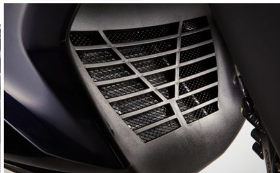
Lower cowling improves engine cooling efficiency
